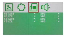
HSTART: Sets the left alignment point of image. HSIZE: Sets the horizontal size of the image. VSTART: Sets the lower alignment point of the image. VSIZE: Sets the vertical size of the image.
