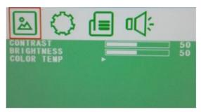
CONTRAST: Sets the contrast of the image (difference between the light and dark areas of the picture) (0–100).
