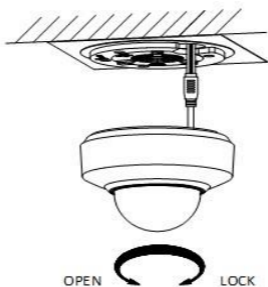
Figure 2-8 Secure the PTZ Camera
